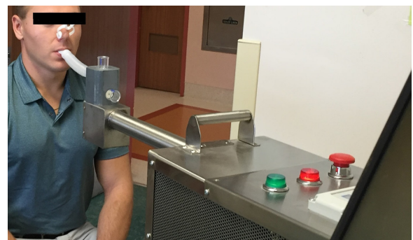
Figure 1. Exhaled breath condensate (EBC) collection device with a nasal clip.
